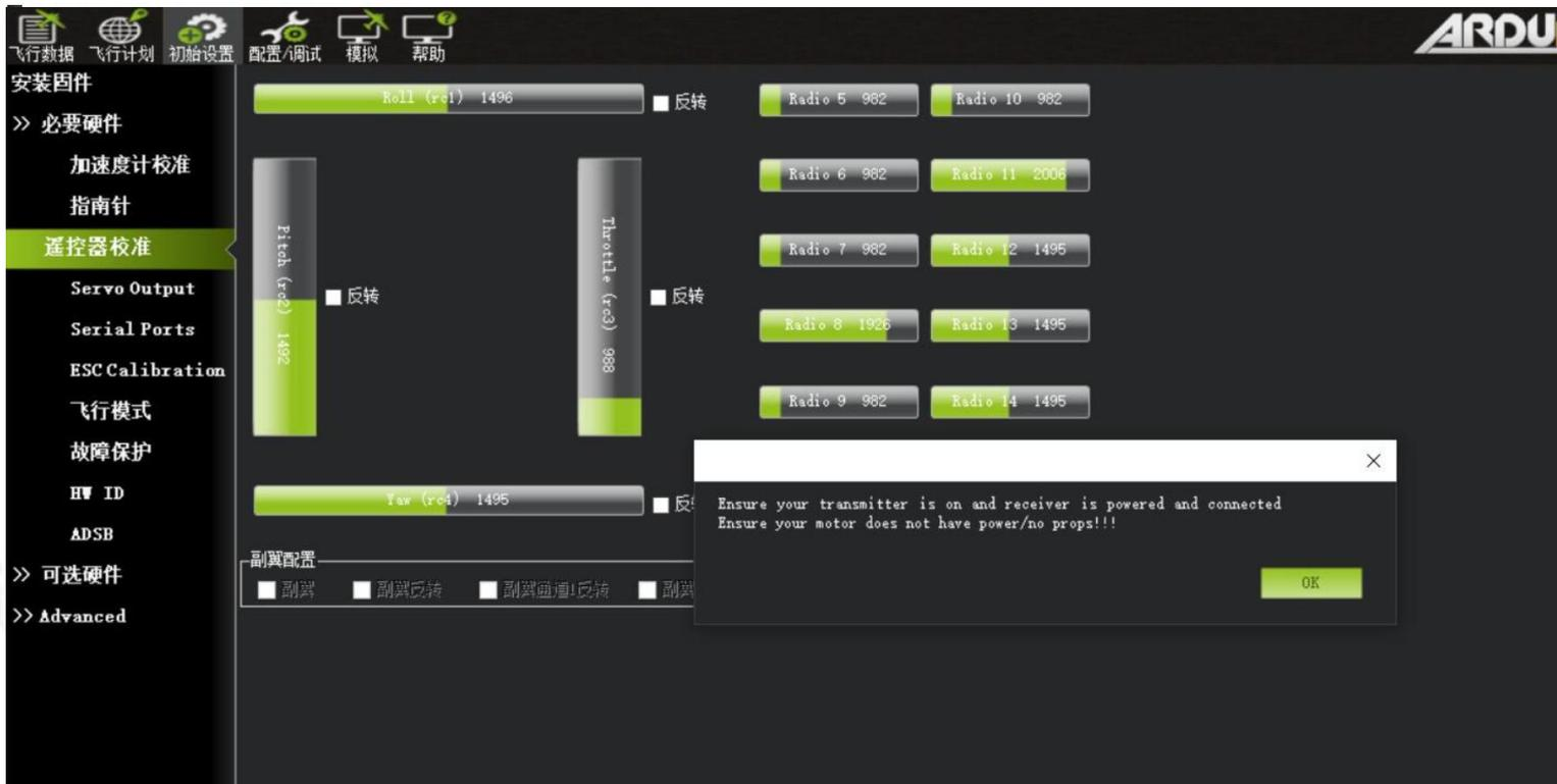
点击“校准遥控”弹出对话框“Ensure your transmitter is on and receiver is powered and connected. Ensure your motor does not have power/no props!!!”旨在提示请确认遥控器油门通道的方向，并确保电机未接电及未安装螺旋桨。点击OK。
